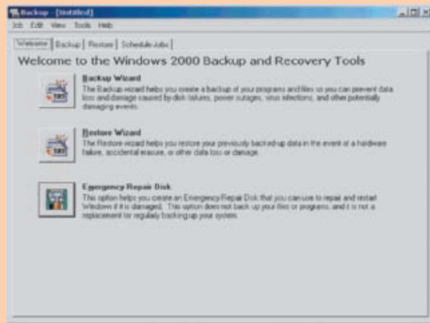
Figure 15-55 Use the Backup window to back up the registry and create an emergency repair disk Courtesy: Course Technology/Cengage Learning
