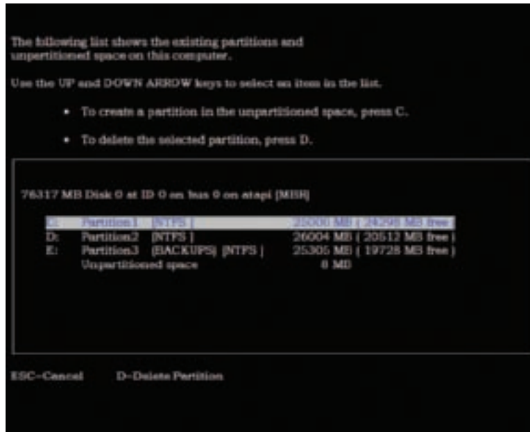
Figure 15-53 Using the Diskpart screen, you can view, delete, and create partitions Courtesy: Course Technology/Cengage Learning
