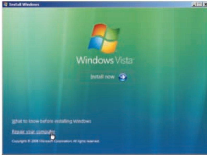
Figure 15-32 Launch Windows RE after booting from the Vista DVD Courtesy: Course Technology/Cengage Learning
