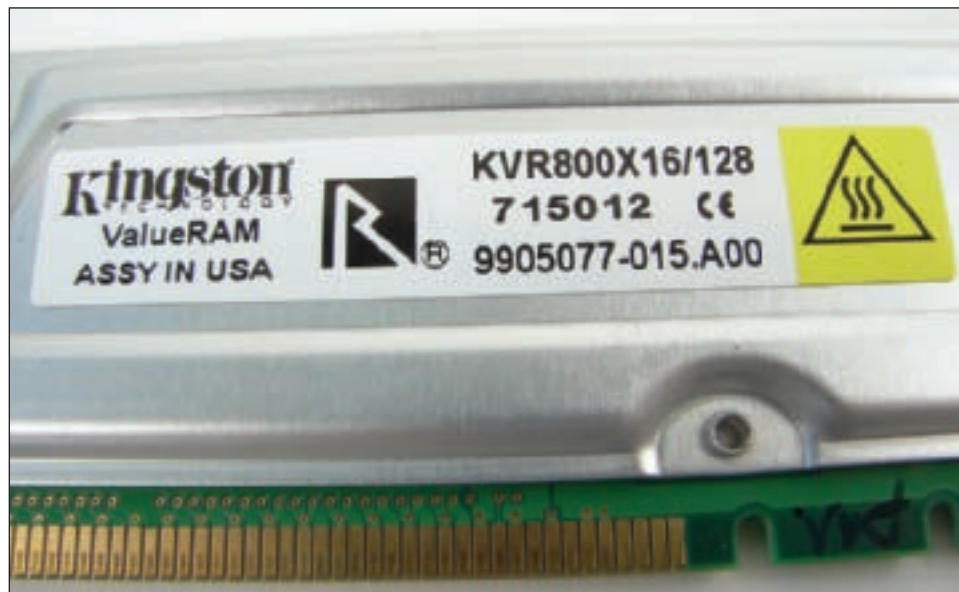
Figure 7-17 Use the label on this RIMM to identify its features Courtesy: Course Technology/Cengage Learning
