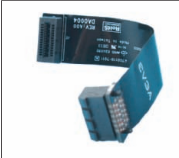
Figure 9-38 SLI bridge connects two SLI video cards Courtesy: Course Technology/Cengage Learning
