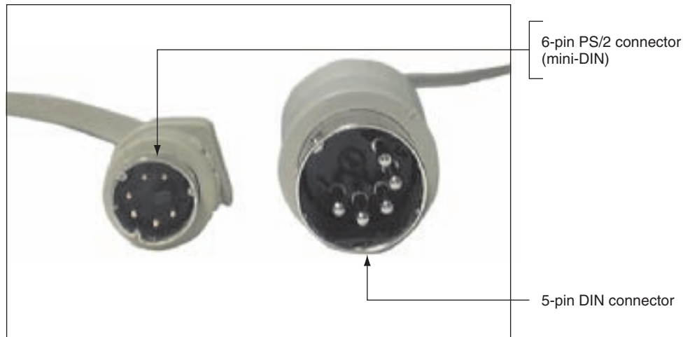
Figure 9-40 Two PS/2 and DIN connectors used by keyboards and mice Courtesy: Course Technology/Cengage Learning
