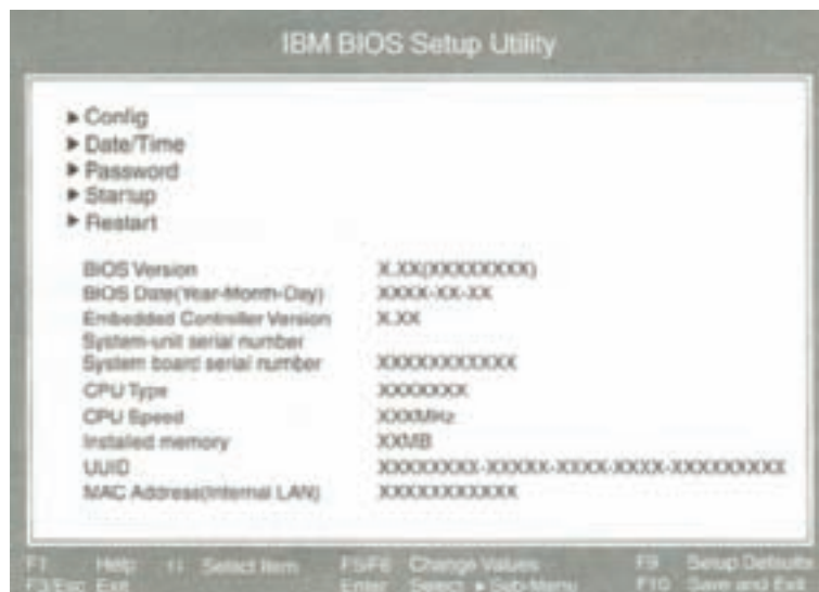
Figure 5-64 BIOS setup main menu for an IBM computer Courtesy: Course Technology/Cengage Learning
