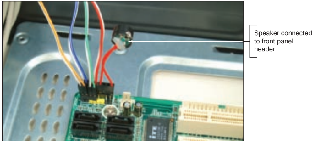
Figure 5-56 Front panel header with all connectors in place Courtesy: Course Technology/Cengage Learning
