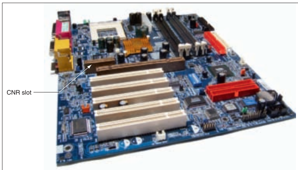
Figure 5-20 A CNR slot is smaller than a PCI slot but about the same height Image copyright 2009, Slobodan Djajic. Used under license from Shutterstock.com
