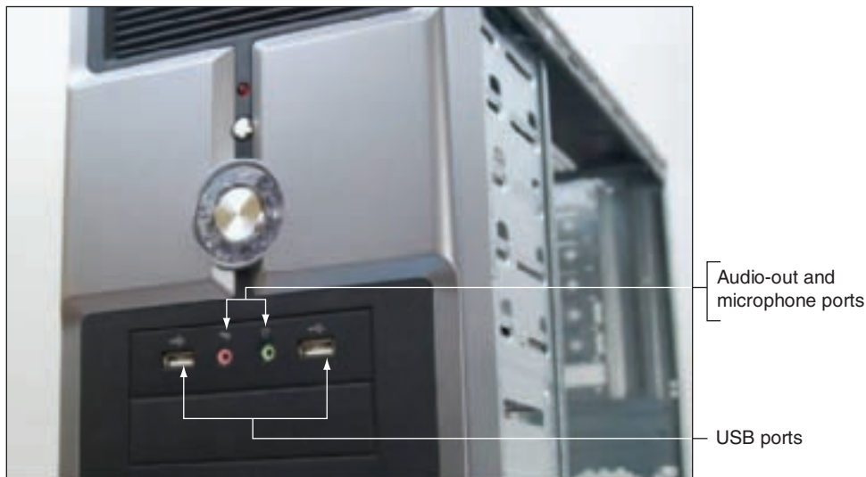
Figure 5-57 Ports on the front of the computer case Courtesy: Course Technology/Cengage Learning
