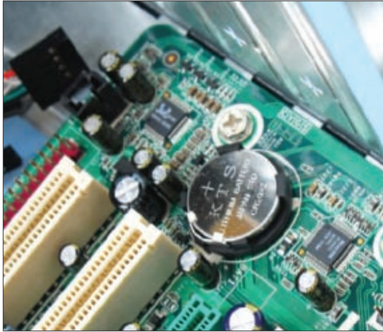
Figure 5-30 The coin-cell battery powers CMOS RAM when the system is turned off Courtesy: Course Technology/Cengage Learning
