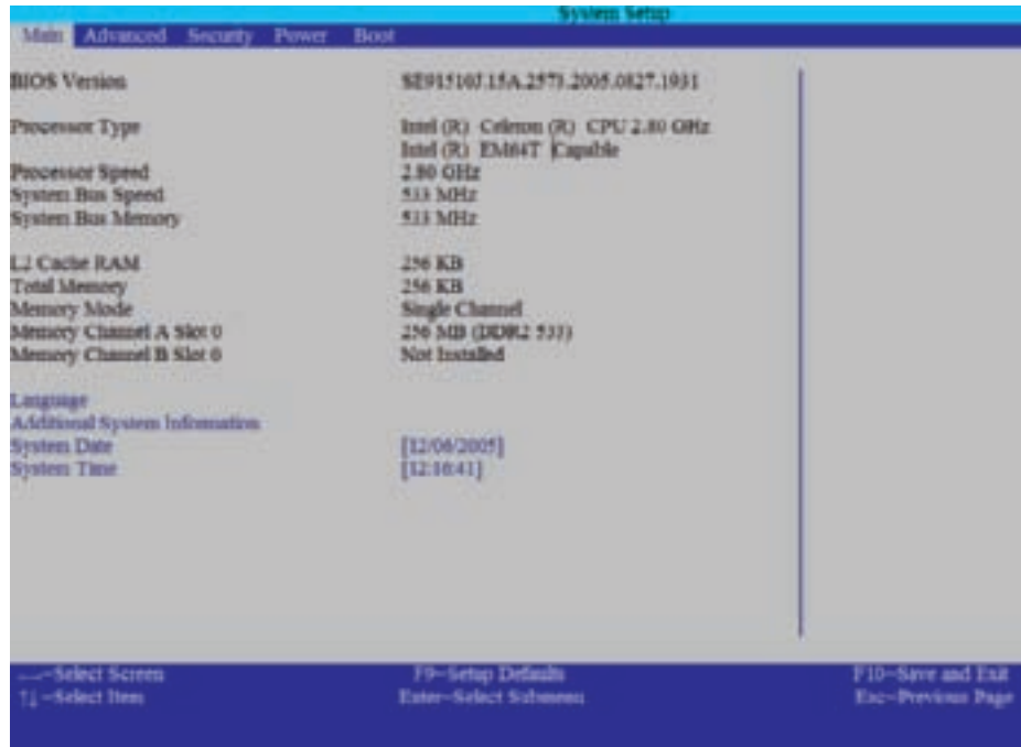
Figure 5-65 BIOS setup main menu for a Gateway computer Courtesy: Course Technology/Cengage Learning
