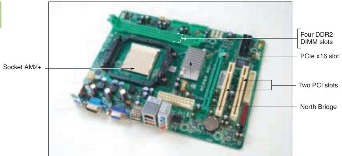
Figure 5-2 This MicroATX motherboard by Biostar has an AM2 socket that supports an AMD processor Courtesy: Course Technology/Cengage Learning
