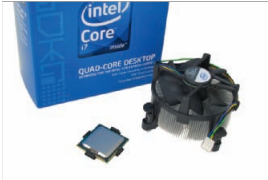
Figure 6-6 The Intel Core i7 processor (processor number i7-920) with boxed cooler Courtesy: Course Technology/Cengage Learning
