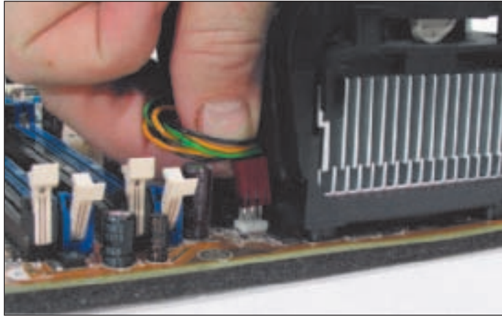
Figure 6-43 Connect the CPU fan power cord to the motherboard fan header Courtesy: Course Technology/Cengage Learning
