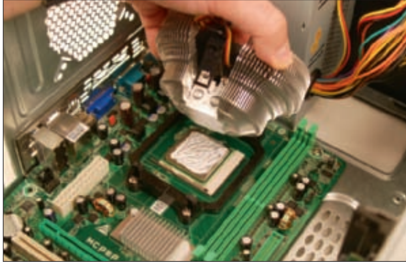
Figure 6-47 Align the cooler over the retention mechanism Courtesy: Course Technology/Cengage Learning
