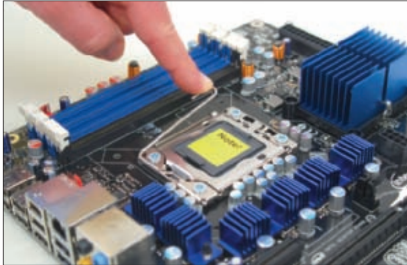
Figure 6-20 Release the lever from the socket Courtesy: Course Technology/Cengage Learning
