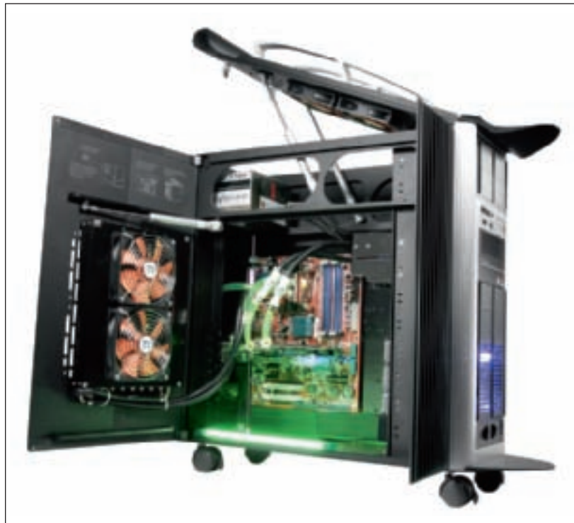
Figure 6-16 A liquid cooling system pumps liquid outside away from components where fans can then cool the liquid Courtesy of Thermaltake (USA) Inc.
