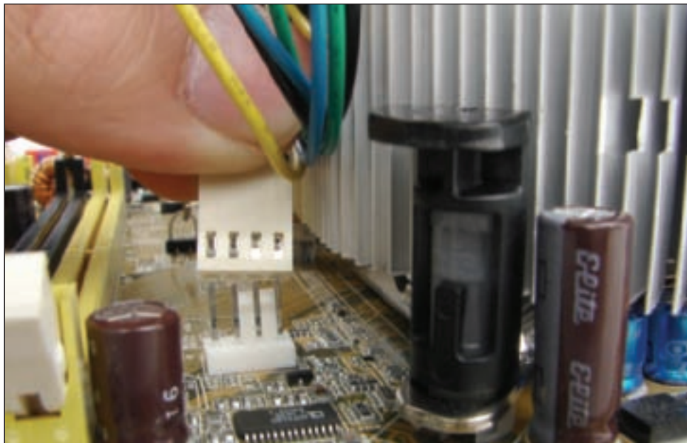
Figure 6-31 Connect the cooler fan power cord to the motherboard CPU fan header Courtesy: Course Technology/Cengage Learning
