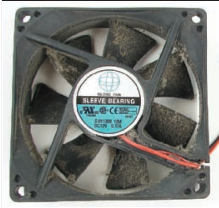
Figure 6-17 This dust-jammed fan caused a system to overheat Courtesy: Course Technology/Cengage Learning
