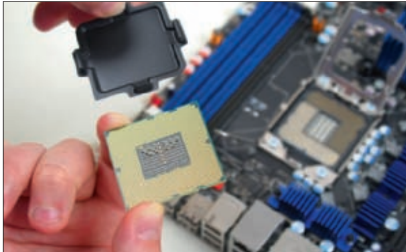
Figure 6-23 Remove the protective cover from the processor Courtesy: Course Technology/Cengage Learning
