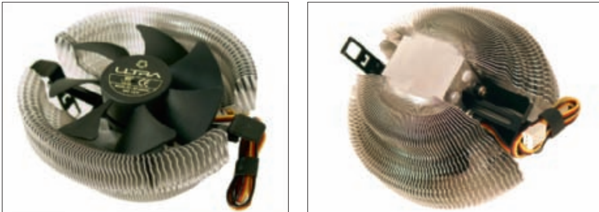
Figure 6-9 A cooler sits on top of a processor to help keep it cool Courtesy: Course Technology/Cengage Learning
