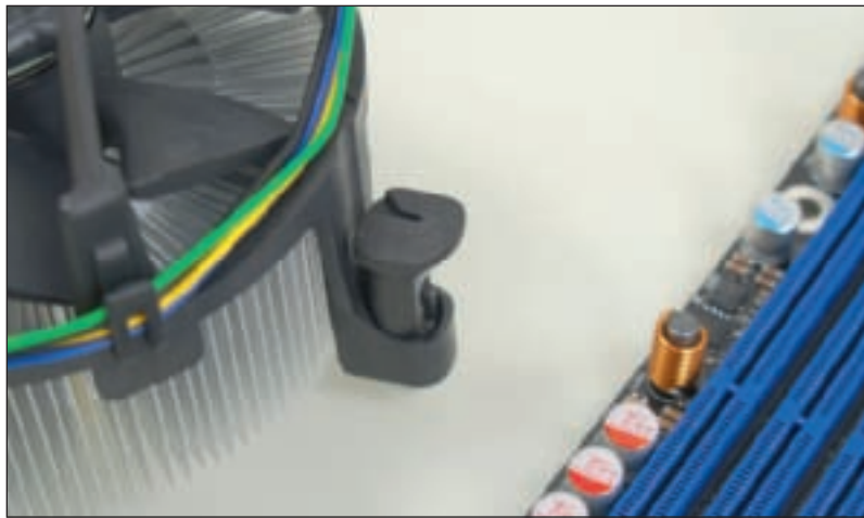
Figure 6-28 Align the locking pins so they are perpendicular to the heat sink Courtesy: Course Technology/Cengage Learning
