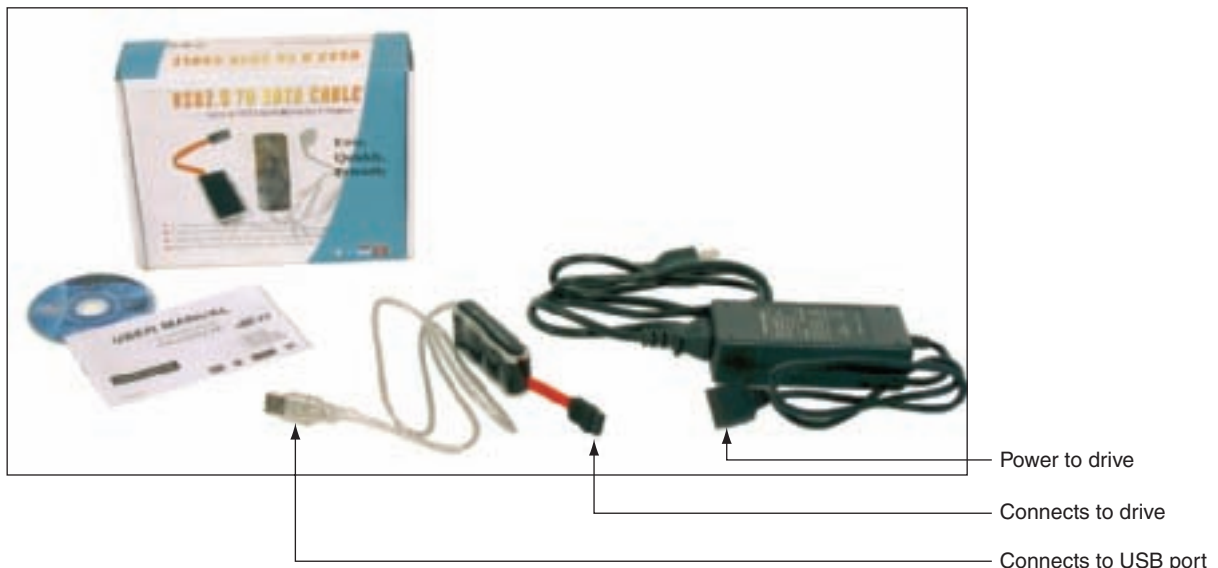
Figure 8-61 Use a SATA to USB converter to recover data from a drive using a SATA connector Courtesy: Course Technology/Cengage Learning
