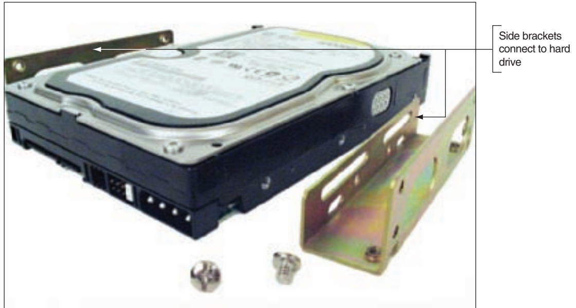
Figure 8-45 Use the universal bay kit to make the drive fit the bay Courtesy: Course Technology/Cengage Learning
