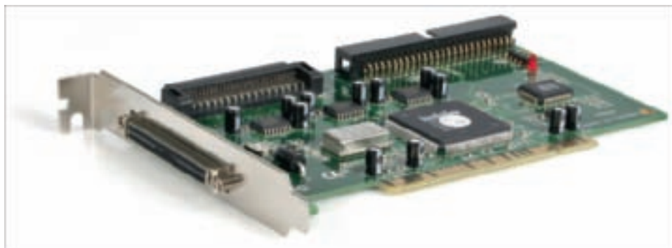
Figure 8-15 PCI SCSI host adapter card by StarTech Courtesy of StarTech.com
