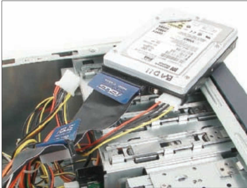
Figure 8-59 Temporarily connect a faulty hard drive to another system to diagnose the problem and try to recover data Courtesy: Course Technology/Cengage Learning
