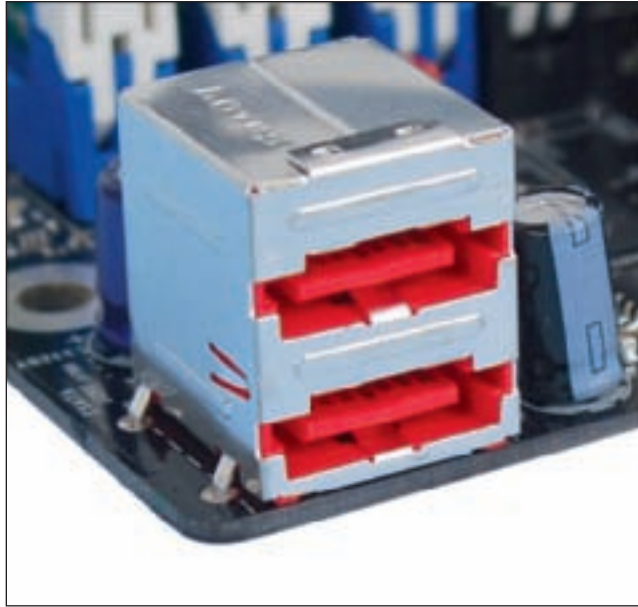
Figure 8-13 Two eSATA ports on a motherboard Courtesy: Course Technology/Cengage Learning
