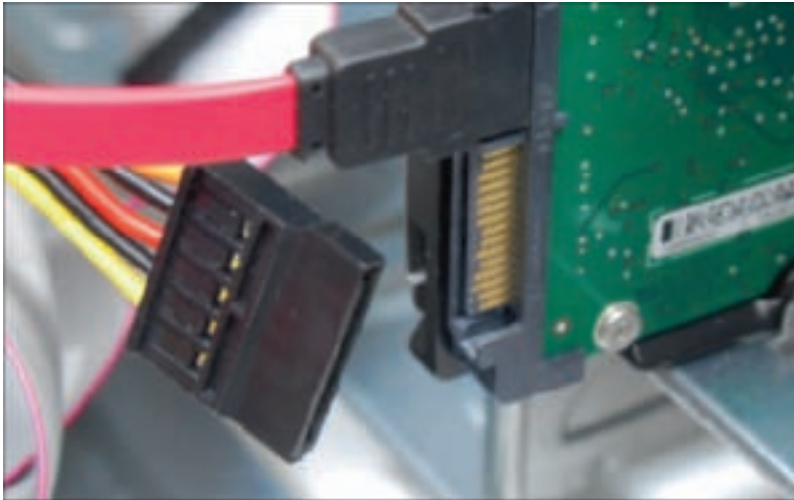
Figure 8-26 Connect the SATA power cord to the drive Courtesy: Course Technology/Cengage Learning
