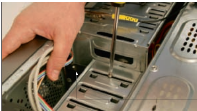
Figure 8-24 Secure the other side of the drive with one or two screws Courtesy: Course Technology/Cengage Learning
