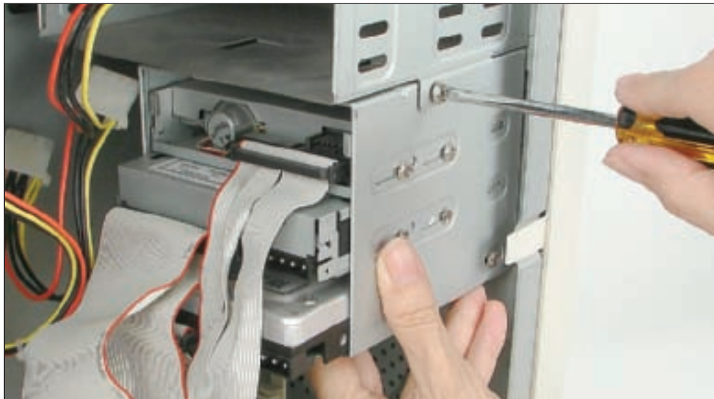
Figure 8-41 Secure the bay with the bay screw Courtesy: Course Technology/Cengage Learning
